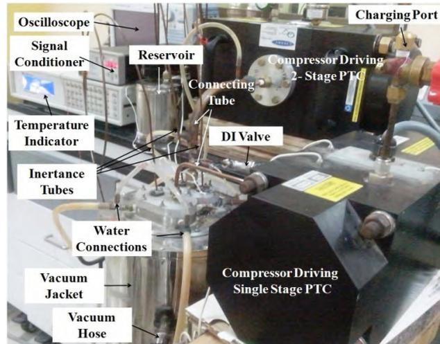
Fig. 2. Experimental setup for three stages thermally coupled PTCs.
