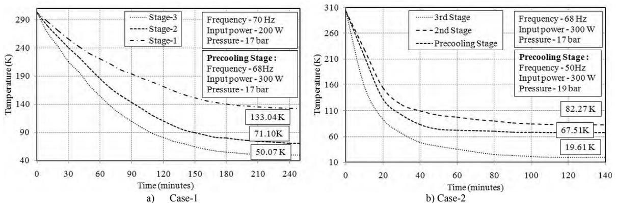
Fig. 3. Cool down curve for three stages thermally coupled PTC.
