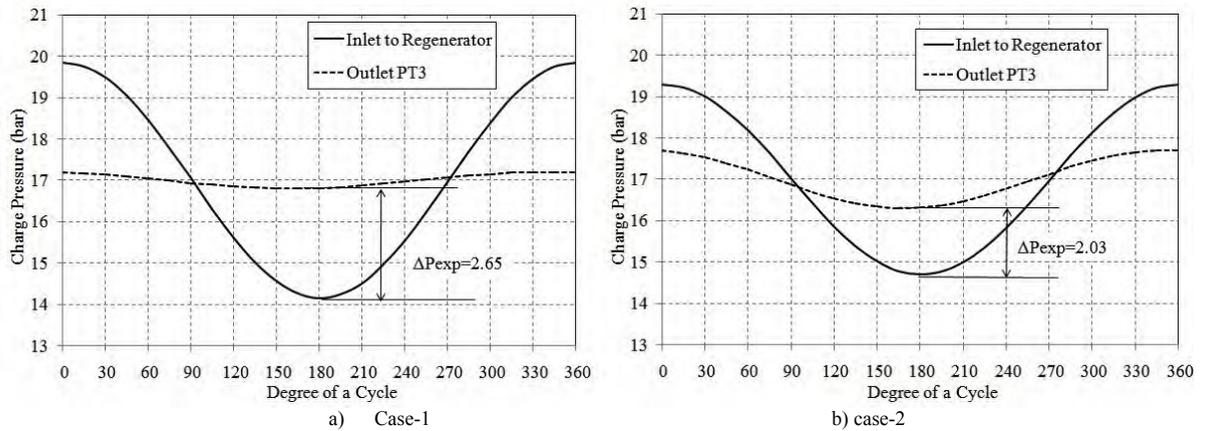
Fig. 4. Pressure variation for three stages thermally coupled PTC case-1.
