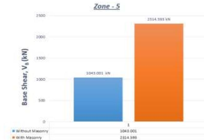
Figure 5 Base Shear Comparison Graph for zone-5 building with/without masonry
