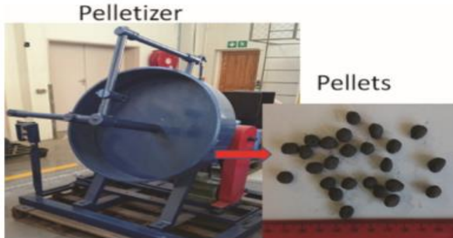
Figure 1 Pelletization of waste gypsum in a disc pelletizer
