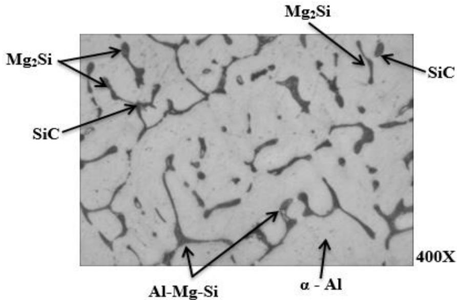
**Figure 5: Presence of SiC, Mg<sub>2</sub>Si and Al-Mg-Si in AA 6351 + 5% SiC observed using Optical Microscopy (OM)**
