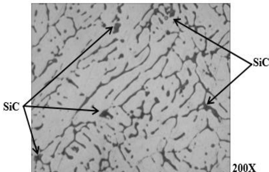
**Figure 4: Optical Microscopy (OM) of AA 6351 + 5% SiC**
