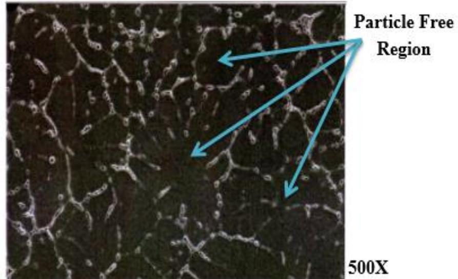
**Figure 6 : SEM Micrograph of AA 6351 + 5% SiC**
