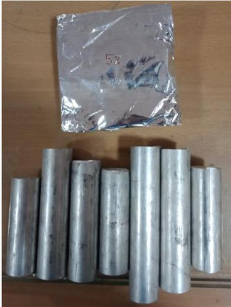
**Figure 2: Aluminium alloy and SiC particles as per weight fraction**
