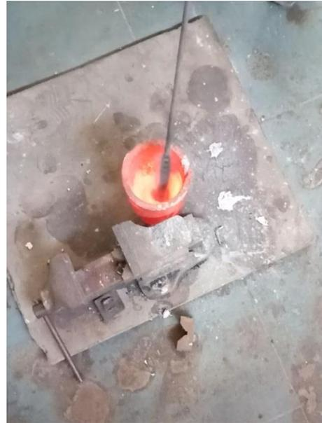
**Figure 3: Stirring of molten composite**
