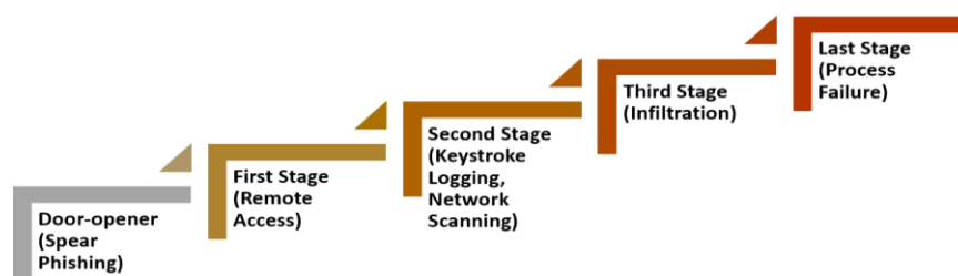
Fig. 7: Security breach stages for a German Steel Facility 26
