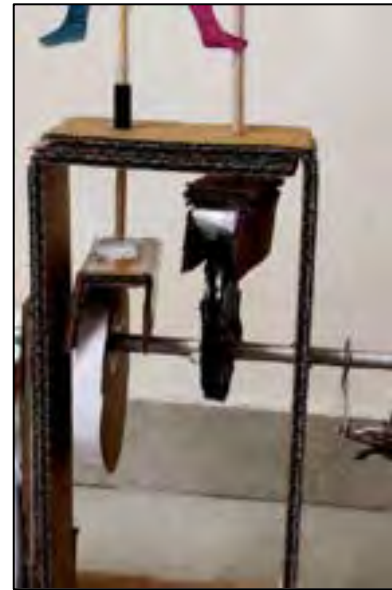
Figure 6: Cam , Shaft and Follower
