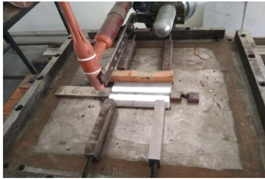
Figure 3: Application of flux before welding
