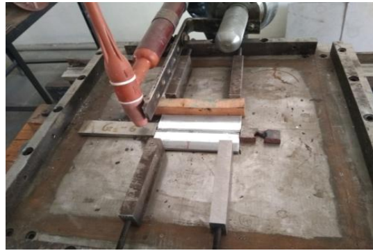
Figure 3: Application of flux before welding
