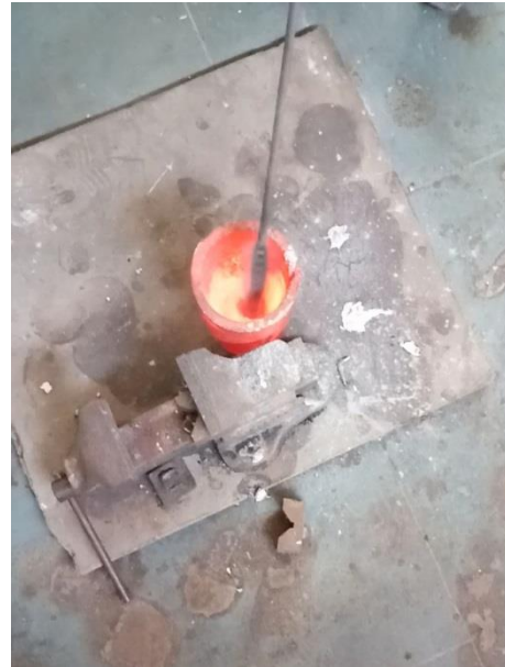
Figure 3: Stirring of molten composite
