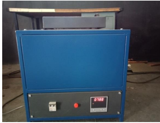
Figure 1: Electrical Furnace used for melting matrix material
